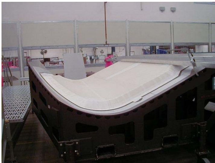
Figure 1. Cured and trimmed test article placed back on process tooling to measure dimensional fidelity.
