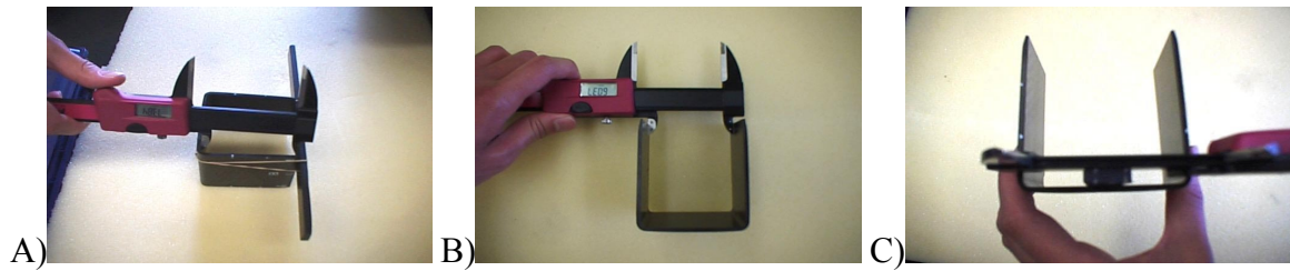
Figure 5. Measurement of: A) section height, H , B) flange-to-flange distance, W , and C) web width, B , on a sectioned rib.
